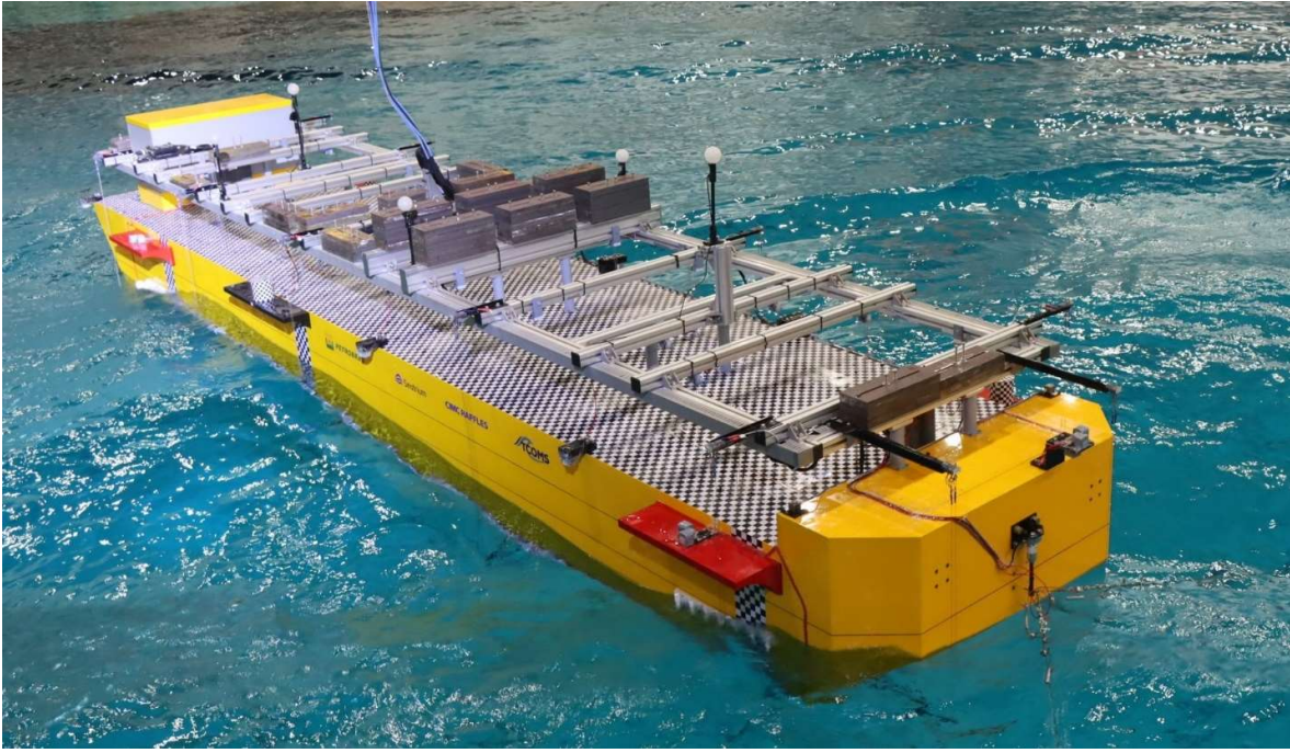
Caption: Scaled model tests undertaken at TCOMS' ocean basin facility to validate the performance of the FPSOs.
